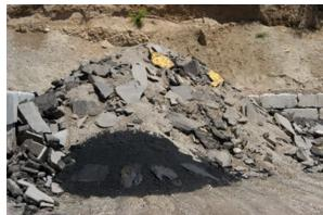
Recycled materials operations are a key component for many contractors in Utah, supplying quality recycled asphalt and concrete, which is used mainly as a road base product for streets, subdivisions and parking lots.
