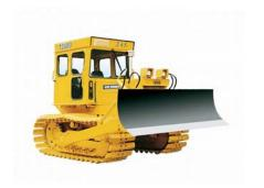
**bulldozer** - a construction vehicle with tracks or large wheels and a wide blade used for moving earth or debris
