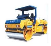
**roller** - a compactor type engineering vehicle used to compact soil, gravel, concrete, or asphalt in the construction of roads and foundations
