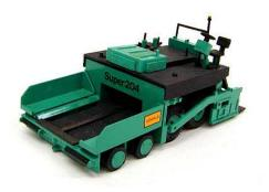
**paving machine** - an engineering vehicle used to lay asphalt on roadways. It is normally fed by a dump truck
