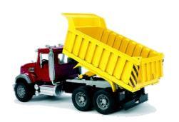
**dump truck** - a heavy truck with an open bed that can be tilted up and back to unload cargo such as gravel, dirt, or refuse from construction sites
