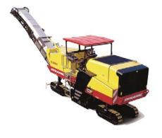
**cold planer** (also known as a pavement planer, pavement recycler, asphalt milling machine or roto-mill) - a construction machine used to remove bituminous pavement or asphalt concrete from roadways, resulting in a somewhat rough, even surface that can be repaved with a smoother surface
